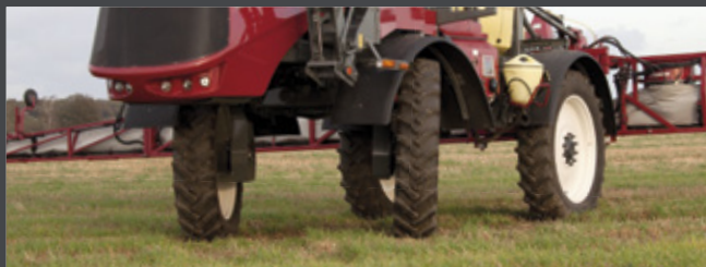
Front wheel steering – road traffic
