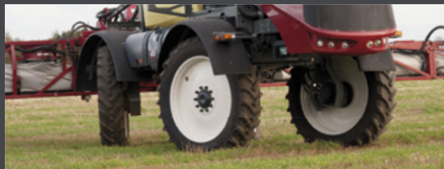
4-wheel steering – field mode
